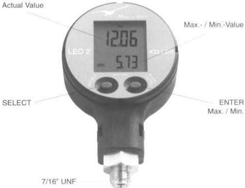
**Figure 5.** Front View Of The Digital Pressure Gauge
