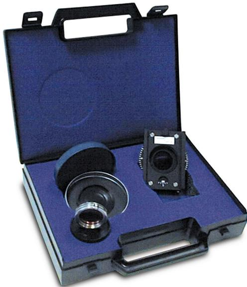
Polarizer Rotator 3" x 2" Slide Mount
