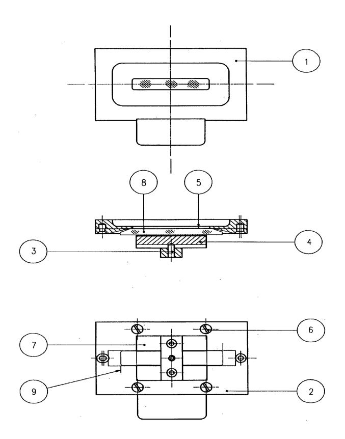
Fig.1: Trough top-plate of P/N 11050 ATR - crystal removal and replacement
