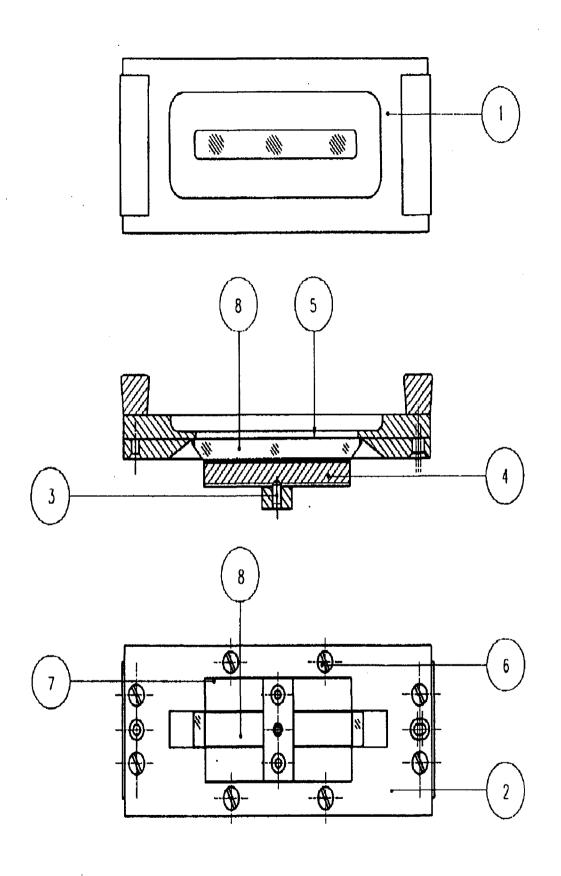
Fig.2: Trough top plate of P/N 1110 and P/N 11160 series ATR - crystal removal and replacement
