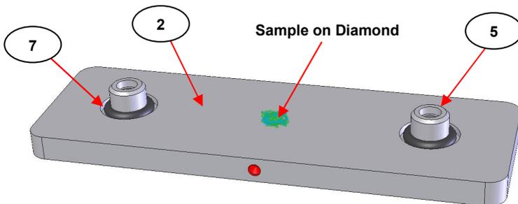
**Fig 4. Sample Placed Over Diamond Window on Lower Support Plate Assembly**
