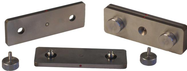
The clear aperture of 1.5 mm diameter offered by the hastalloy plate allows for a good transmission throughput signal when placed at the sampling focus of an FTIR spectrophotometer using an MCT detector. For optimum performance with a DTGS detector, the Microfocus Beam Condenser P/N GS02560 (with ZnSe lenses) or P/N GS02561 (with KRS-5 lenses) is recommended to be used with the DC-3 in order to obtain high quality spectra.
