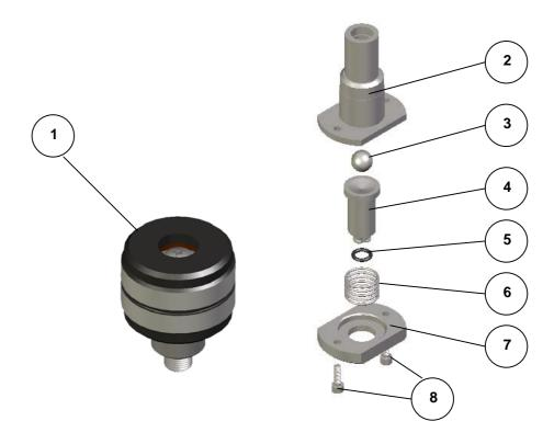
The parts (3) through to (8) are retained from the original bridge pieces of the Golden Gate ATR accessory.
