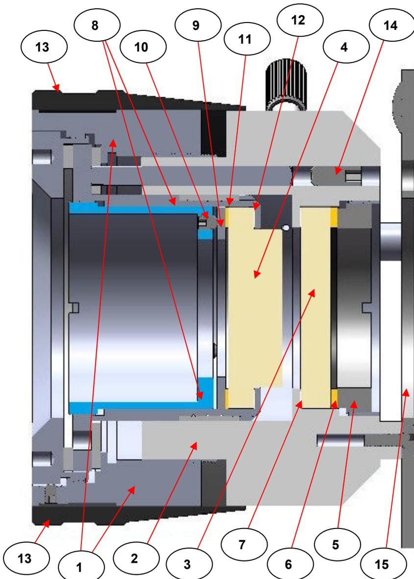
**Fig 2. Cutaway Side View of Variable Pathlength Liquid Cell GS07500 Series**
