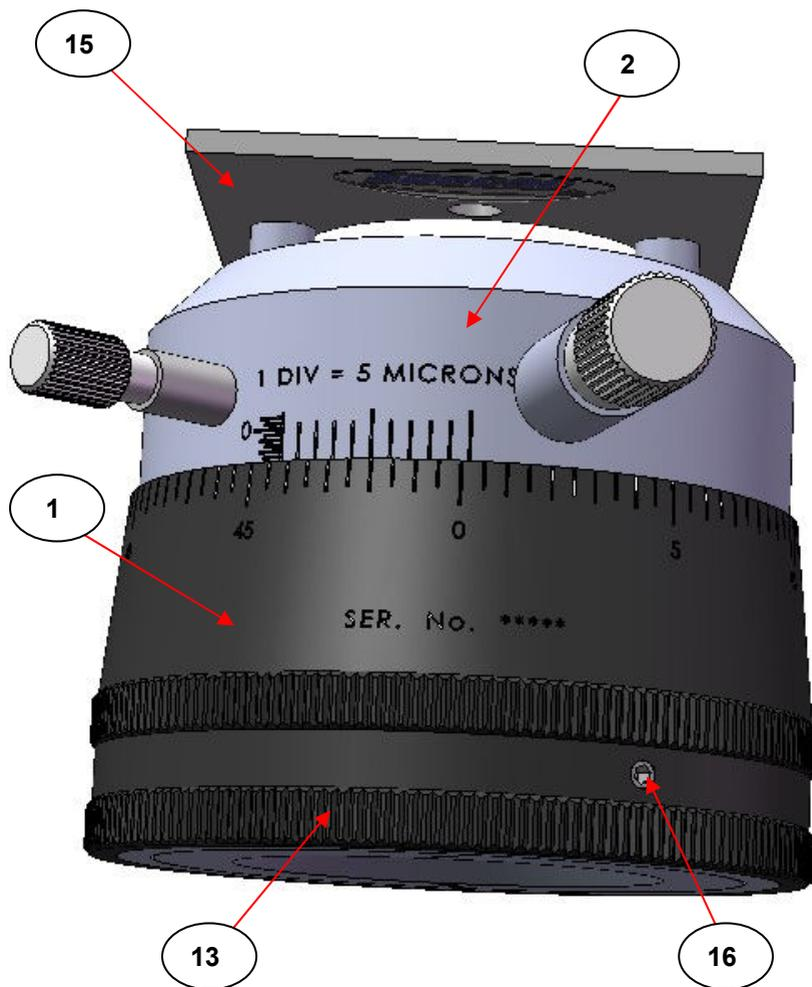
**Fig 1. View of Vernier Scales for Pathlength Setting of the Variable Pathlength Liquid Cell GS07500 Series**
