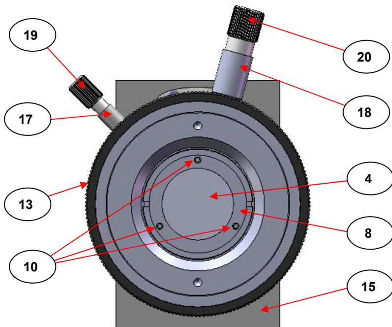
**Fig 4. Front View of the Variable Pathlength Cell GS07500 Series**
