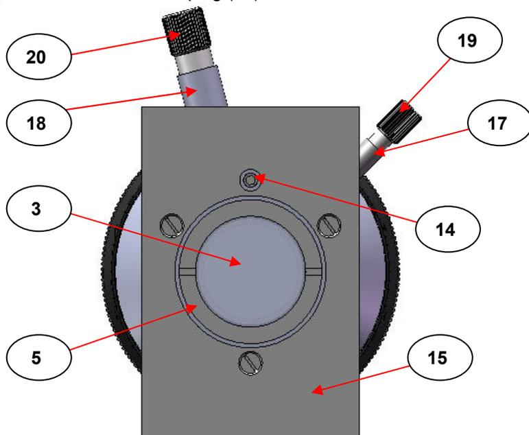
**Fig 5. Back View (Through 3" x 2" Mount Plate) of the Variable Pathlength Cell GS07500 Series.**
