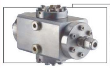
Specac flow cells can operate at temperatures as high as 280°c and pressures as high as 1500 p.s.i. A choice of body materials, including Stainless Steel 316L and Hastelloy® C276 are available to ensure materials compatibility with a wide range of process fluids. Special materials are available upon request.
